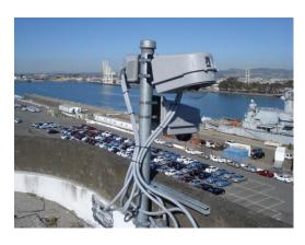
Over 100 Axis Megapixel IP cameras are installed in city part and port area. With wireless mesh technology from Belair, the live images can travel across the city, and back to the integration system of GVD in the police office as the control centre, and GVD's storage system supports to save all images up to 6 months. It will be a powerful resource
